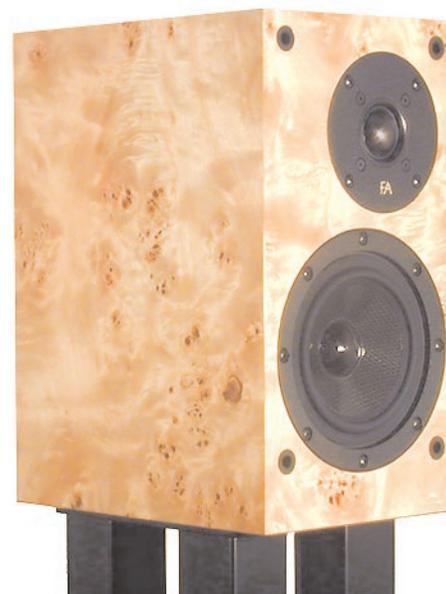
soft dome tweeter in a 13 inches (H) by 7 inches (W) by 1 inch (D) cabinet, weighing in at 20 pounds. Frequency response is listed as 45 Hz - 22 kHz,  $\pm 3$  dB, and sensitivity is rated at 85 dB at 1 watt/1 meter. Impedance is 8 ohms, recommended power is 20 - 200 watts. The custom-designed crossover sits at 2.7 kHz. The particular set I have been auditioning has a Piano Walnut finish, but it is also available in Burr Oak and black.
