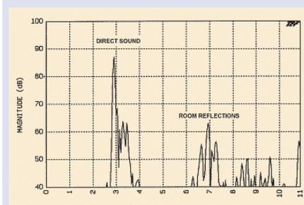
In **Figure 2** is the Energy Time Curve, which correlates with the transient response. The time scale is 11 msec. We see an extremely sharp direct-sound spike with delayed vibrations about 25 dB down.
