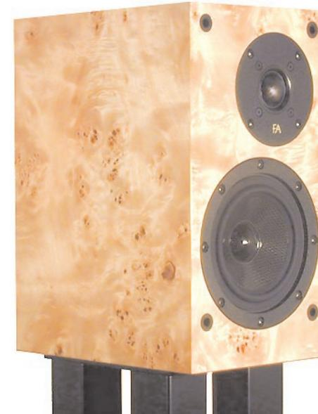
soft dome tweeter in a 13 inches (H) by 7 inches (W) by 1 inch (D) cabinet, weighing in at 20 pounds. Frequency response is listed as 45 Hz - 22 kHz,  $\pm 3$  dB, and sensitivity is rated at 85 dB at 1 watt/1 meter. Impedance is 8 ohms, recommended power is 20 - 200 watts. The custom-designed crossover sits at 2.7 kHz. The particular set I have been auditioning has a Piano Walnut finish, but it is also available in Burr Oak and black.
