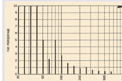
Finally, **Figure 3** shows the Total Harmonic Distortion vs. frequency at 90 dB SPL, 1 meter. It is very good for such a small speaker: below audibility from 100 Hz up, THD reaches 5% at 50 Hz and 80 Hz. If the FS68 were used with a subwoofer, that distortion could be reduced by high-pass filtering the signal driving the FS68. During the THD test, the rear-port tube buzzed slightly, which may have influenced the measurement.
